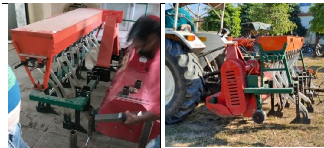
Fig 3.14 Nine row mulcher cum seed drill
