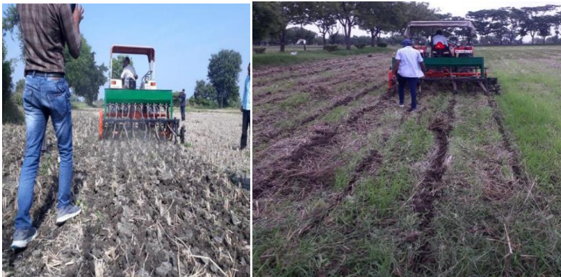
Fig 3.15 Sowing of wheat and maize with slit till drill
