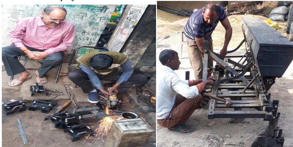
Fig 3.19 Fitting of inverted T type furrow openers in seed cum fertilizer drill
